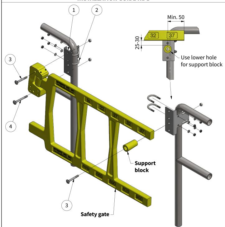
Supplied with U-bolts suitable for 42-48 mm pipe. In case of other diameters please contact us; we supply U-bolts for pipe sizes 30-76 mm.
